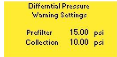
Figure 7.4.2 Filter Differential Pressure Screen
